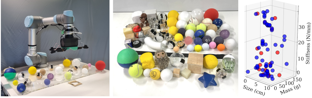
Figure 2: Robot with UR5 arm, customized Reflex Takkile 2 hand, and wrist-mounted KMS 40 six-axis force-torque sensor (left). The set of 74 objects (including empty space) used for the study with the test set below the black divider (center). The distribution of manually measured object properties: size, mass, and stiffness, with the test set in red (right).
